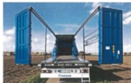
Tautliner, adjustable width Maximum width 3000 mm
